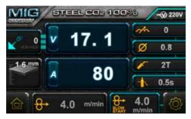
To adjust the voltage independently, Rotate Left Knob (1) to adjust the welding voltage. This will change and give the display screen as below.
