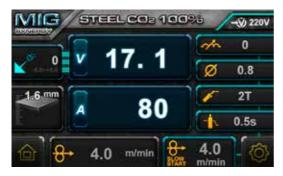
2T/4T function: press the Right Button (4) ,2T/4T Selection Switch to move between 2T and 4T modes. 4T operation means the trigger is pulled once to start welding and pulled again to stop. This is useful for long weld joints. 2T mode, the trigger must be depressed and held during welding.
