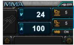
Wire check function: press the Right Button (4) again to enter to the wire check mode, rotate Right knob (3) to select ON/OFF
