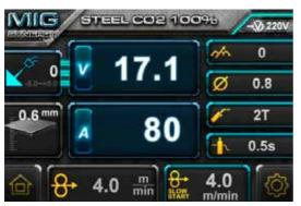
A quick note regarding inductance – this effectively adjusts the intensity of the welding arc. inductance makes the arc 'softer', with less weld spatter. Higher inductance gives a stronger driving arc which can increase penetration. Optimum inductance settings are affected by many welding variables such as: material type, shielding gas joint type, welding amperage, wire size.
