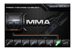
When welding the display will change to show actual welding volts and amperage.
