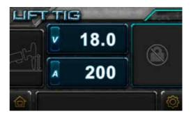
The screen will show the preset LIFT TIG welding current. This can be adjusted by rotating the Right Knob (3)
